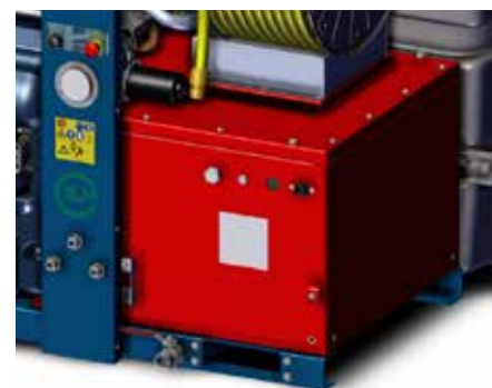
17.6 kW lithium batteries. Autonomy 3300 lt at full power. Recharge 0-100% in 3 hours (400V). Normal 220V charging available. Battery charger on request. Batterie al litio 17.6 Kw. Autonomia massima 3300 lt a piena potenza. Ricarica 0-100% in 3.5 ore (400V). Disponibile 220V carica normale. Caricabatteria optional.
